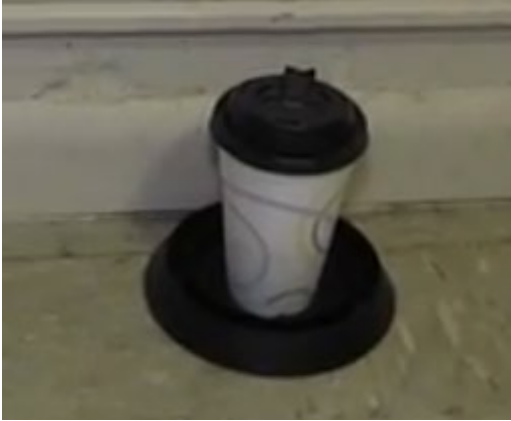
Fig. 5. The dry ice trap consisted of dry ice placed in an insulated coffee cup, and the cup's tab pulled back to let the carbon dioxide slowly escape. The trap sits in a Bedbug Blackout Detector.
