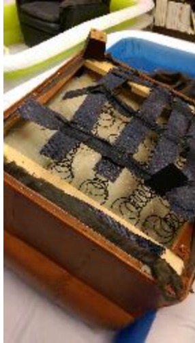
Figure 11. Removing a dust cover provides access to the interior of the furniture, but ensure it's not part of the chair's support system before doing so.
