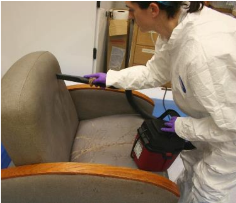
Fig. 3. Rachel demonstrating the vacuuming technique on a hospital bed from a previous study. Note the stocking under the crevice tool.
