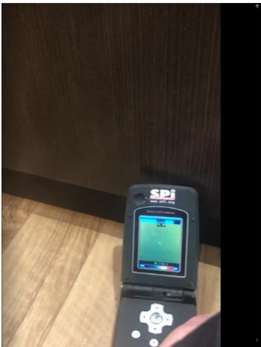
Figure 10. Infrared camera not detecting a hot spot.
