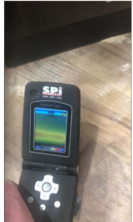
Figure 11. A portable electric heater placed inside the cabinet helped heat penetrate the void created by termite feeding and allowed detection by the infrared camera. The red showing from the kick plate area indicates this area was hotter than surrounding areas and that the drywood termites had probably eaten this wood.
